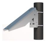
Single-Arm Side Mount easily attaches to poles 2" to 4" in diameter, walls and other flat surfaces, and supports module widths between 5.26" and 25.5", and a tilt range of 15 - 65 degrees. These units are manufactured using heavy-duty corrosion-resistant 5052-H32 aluminum
